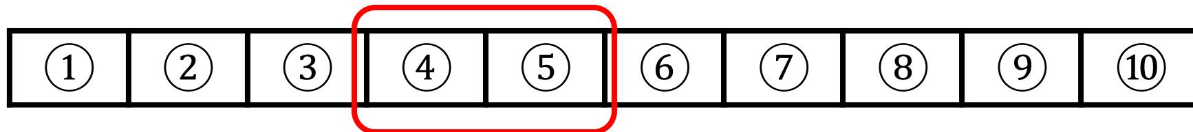
$$\text{Hash}_5 = ① * \text{base}^4 + ② * \text{base}^3 + ③ * \text{base}^2 + ④ * \text{base}^1 + ⑤ * \text{base}^0$$
