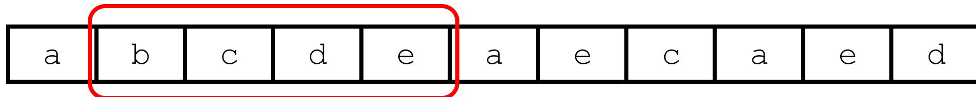
$$\text{Hash1} = a * \text{base}^3 + b * \text{base}^2 + c * \text{base}^1 + d * \text{base}^0$$
