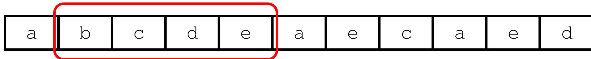
**Hash1** =  $a * \text{base}^3 + b * \text{base}^2 + c * \text{base}^1 + d * \text{base}^0$
